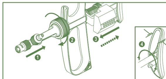
Connect body in pushed position. Adjust magnet orientation to that of counter, holding plunger rod motionless ④.
