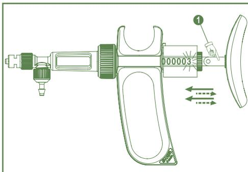
Activate plunger, each shot will increment counter figure if position ① chosen.
